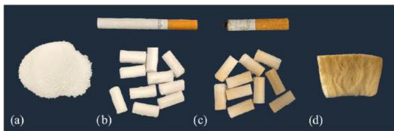
Figure 1. Materials used in leaching experiments: (a) cellulose acetate powder, (b) unsmoked cigarette filters, (c) smoked cigarette filters, and an (d) unraveled (smoked) cigarette filter.
